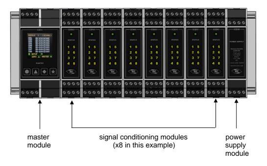
According to the mix of signal conditioning modules, the Iceni node manages the measurement and generation of electrical signals to/from sensors and field devices. Information is exchanged with other nodes in a system via a field communications network connected to the Iceni master module.
