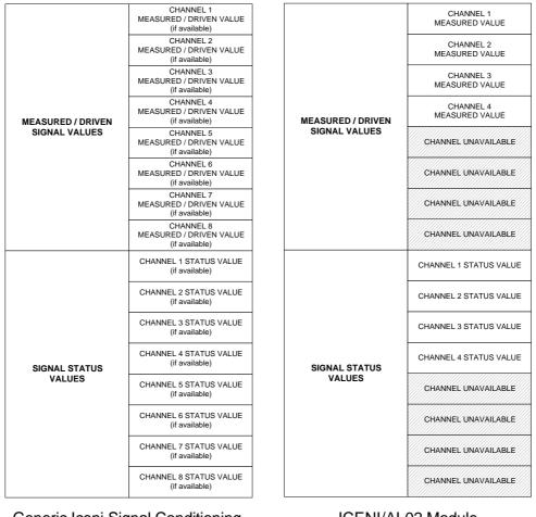
Generic Iceni Signal Conditioning Module Process Image ICENI/AI-02 Module Process Image
