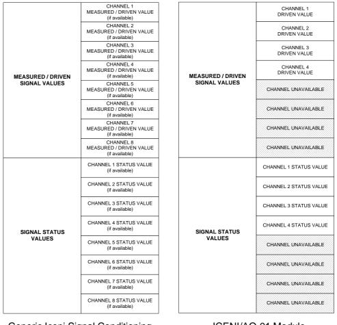
Generic Iceni Signal Conditioning Module Process Image ICENI/AO-01 Module Process Image
