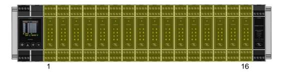
Modules should be assembled with population starting at position 1 on the left hand side, continuing towards position 16 on the right.
