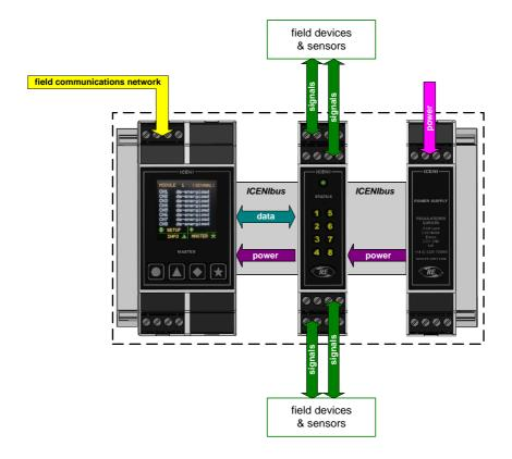
All modules have a 10-way ICENIbus connector on both sides of the lower housing, although for end modules (master and main power supply) one side connector will be supplied fitted with a protective cover.
