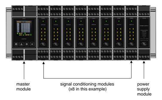
According to the mix of signal conditioning modules, the Iceni node manages the measurement and generation of electrical signals to/from sensors and field devices. Information is exchanged with other nodes in a system via a field communications network connected to the Iceni master module.
